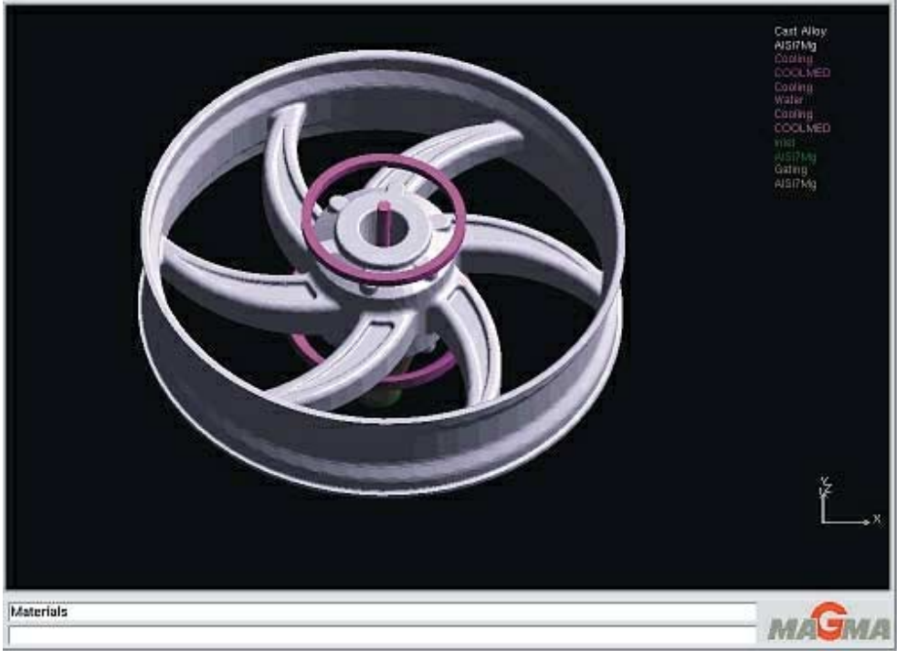
Figure 15: First tempering system proposal in the bottom core with annular cooling as well as point cooling in the hub region
