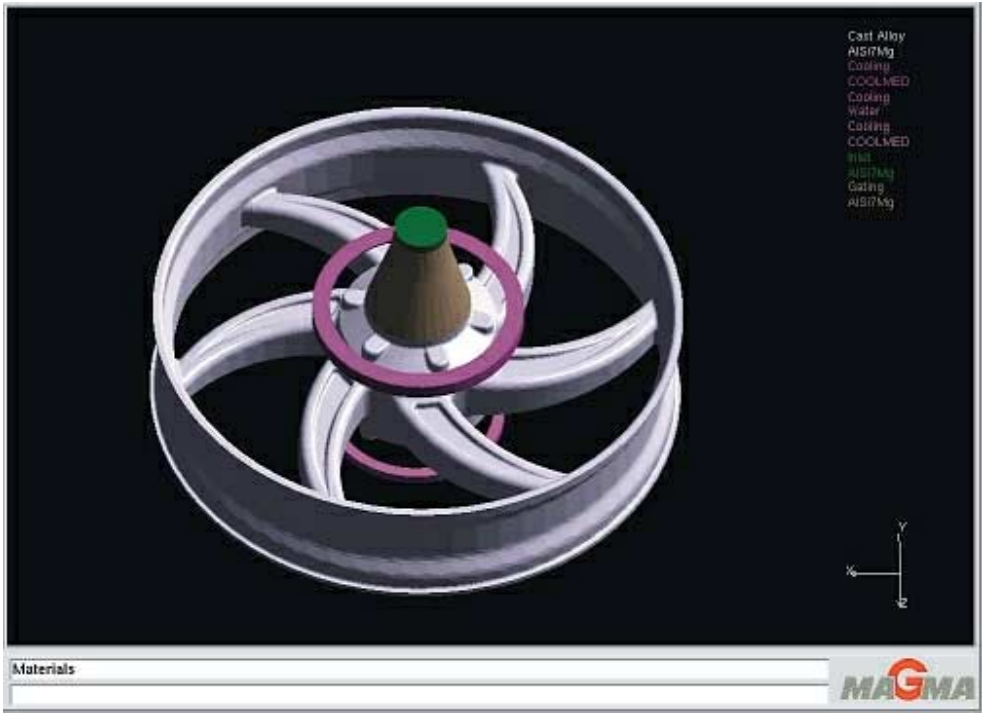
Figure 16: First tempering system proposal in the top core with annular cooling in the gate region
