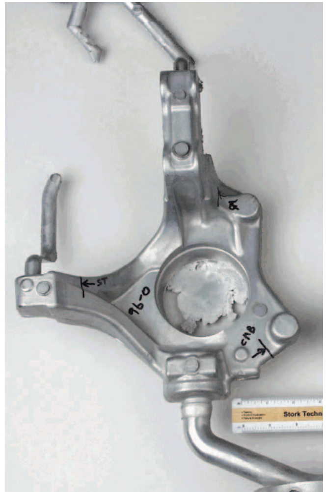
Figure 15 – Prototyped knuckle casting made via the rheocasting process. Several parts were cast for testing and engineering analysis.
