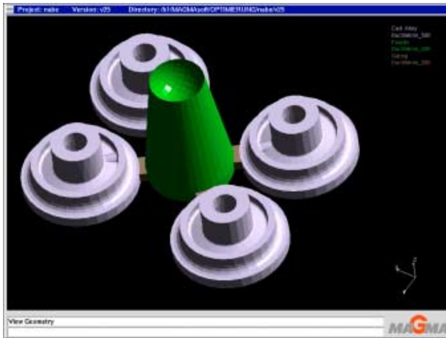
Figure 7: The castings' positions around the central feeder. The quality-relevant area with the thick spot is aligned towards the feeder.
